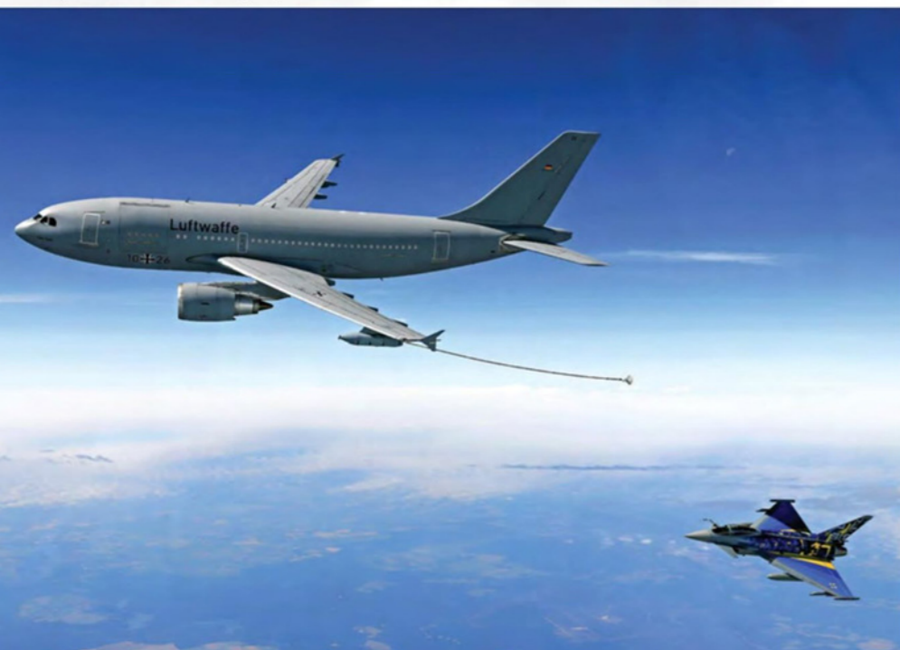
Above: After 15 years of service, the 73 Tactical Air Force Wing is justly proud of the aircraft's 'Carbon Warrior' livery Below: The special Eurofighter undergoes refuelling with a Luftwaffe A310 MRTT (Multi-Role Tanker Transport)
